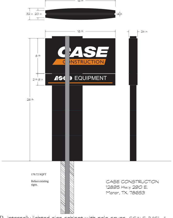
LED internally lighted sign cabinet with pole cover SCALE: 3/16" = 1'
