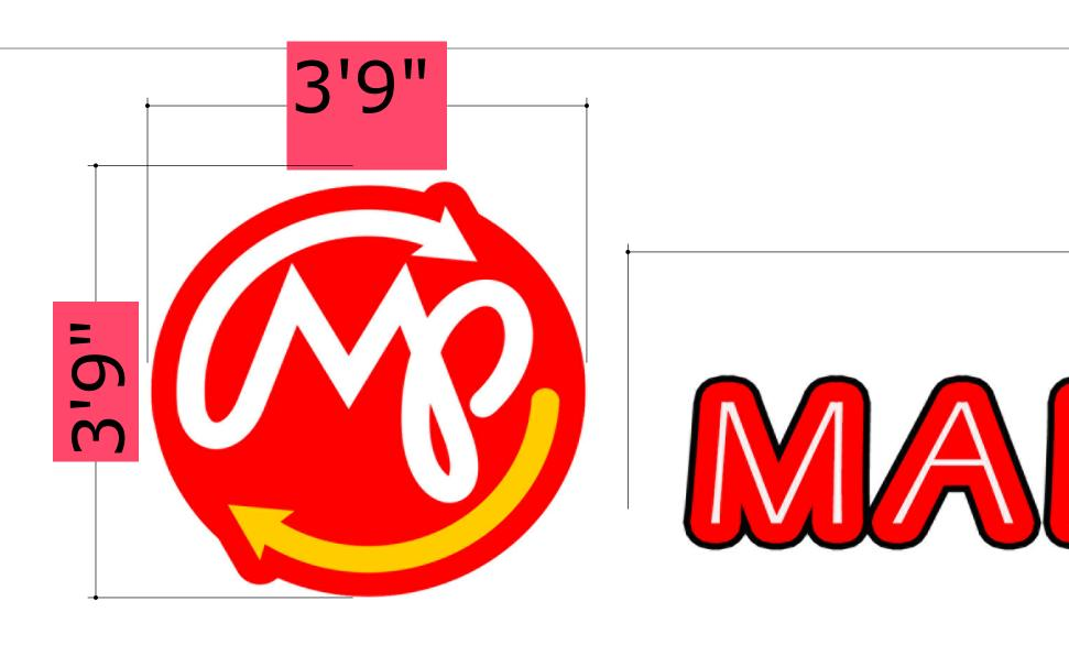
SIGN#1 Size: 3' x 3' x 3" Faces: 1/8" acrylic Face color: Red, Yellow, White Returns: .080 aluminum Return color: Black Voltage: 120vac/12vdc Led Modular: 5000K Mounting: 2" standoff to wall Anchors: 1/4" x 6" studs
