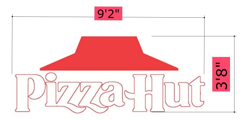
SIGN#6 Size: 9'2" x 3'8" x 3" Faces: 1/8" acrylic Face color: Red,Yellow,White Returns: .080 aluminum Return color: Black Voltage: 120vac/12vdc Led Modular: 5000K Mounting: 2" standoff to wall Anchors: 1/4" x 6" studs
