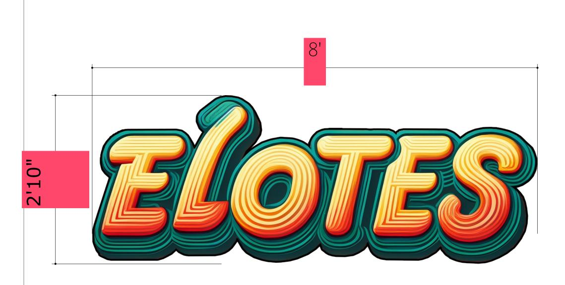
SIGN#5 Size: 8' x 2'10" x 3" Faces: 1/8" acrylic Face color: Red,Yellow, Green Returns: .080 aluminum Return color: Black Voltage: 120vac/12vdc Led Modular: 5000K Mounting: 2" standoff to wall Anchors: 1/4" x 6" studs
