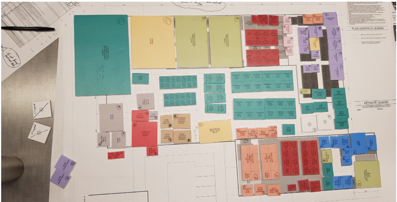
photo of 'Blocking Exercise' from Austin PD Canyon Creek Substation identifying work flow and adjacencies
