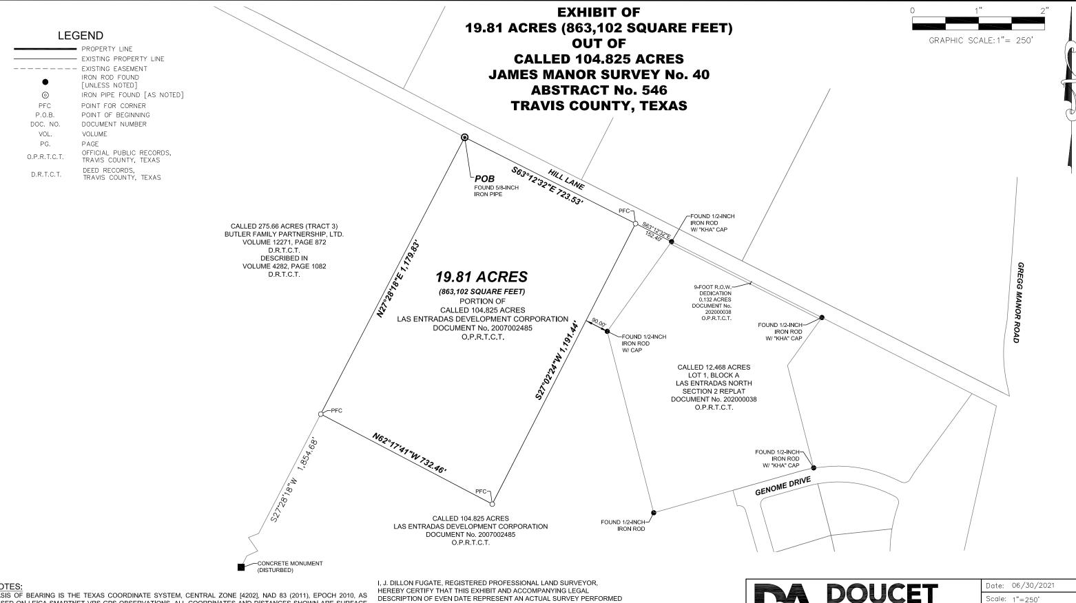
BASIS OF BEARING IS THE TEXAS COORDINATE SYSTEM, CENTRAL ZONE [4202], NAD 83 (2011), EPOCH 2010, AS BASED ON LEICA SMARTNET VRS GPS OBSERVATIONS. ALL COORDINATES AND DISTANCES SHOWN ARE SURFACE VALUES AND MAY BE CONVERTED TO GRID BY USING THE SURFACE ADJUSTMENT FACTOR OF 0.99993 UNITS: US SURVEY FEET
