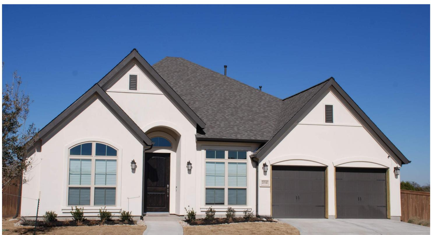
Simple roof lines are encouraged and can be achieved by including hips, gables, projections (e.g. dormers) and roof form changes in keeping with a selected architectural style. On buildings with pitched roofs, the minimum main roof pitch is 5:12. Lower roof pitches are acceptable on porch elements, awnings or architectural feature elements.
