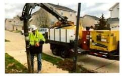
HYDRAULIC BOOM (OPTION). The hydraulic boom offers a 6-way function, wireless remote with vacuum valve operation, 330-degree rotation, remote water jet for ease of cleanout, and a 5-in (13-cm) hose with quick connect to 4-in (10-cm) tooling.
