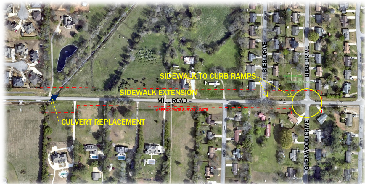
FIGURE 1 – MILL ROAD CULVERT REPLACEMENT AND SIDEWALK EXTENSION
