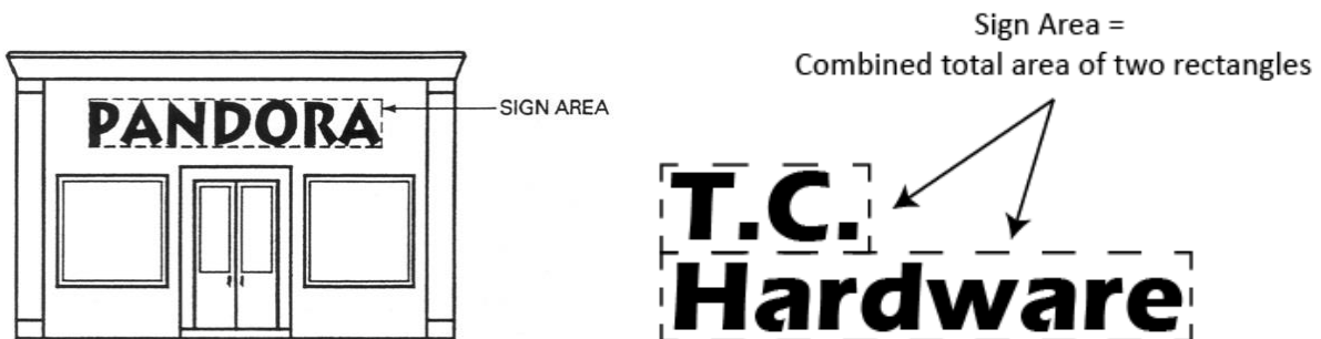
Figure C: Illustration of sign area calculation for two differently shaped wall signs with individual letters.
