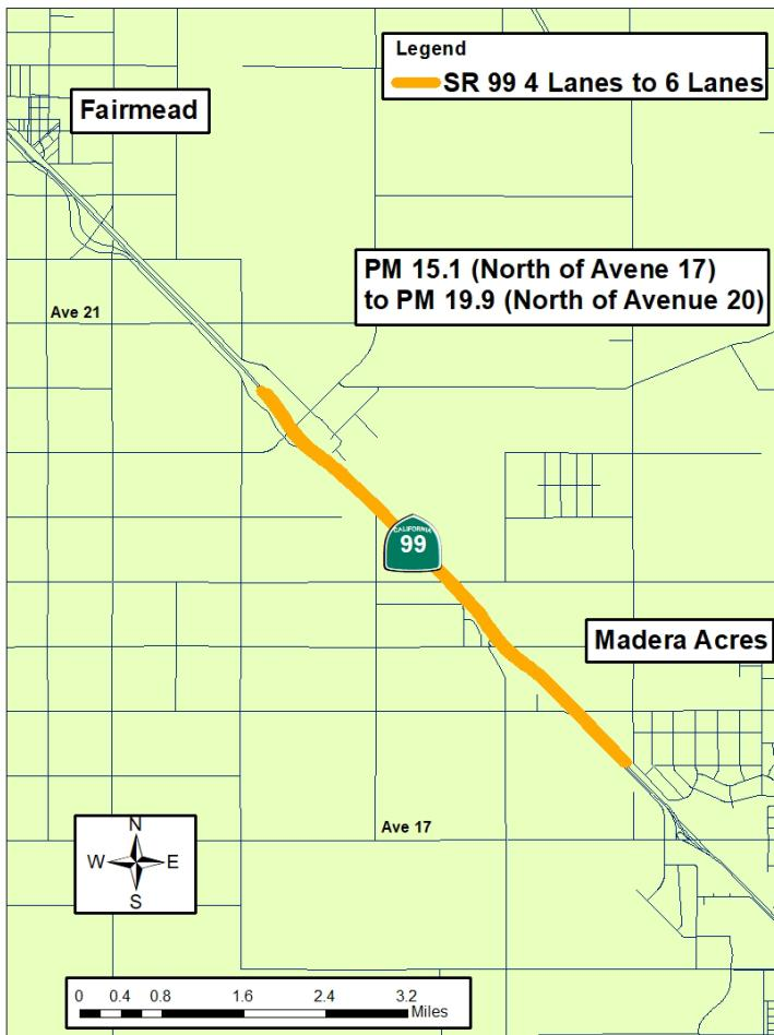
The North Madera SR 99 6 Lane Project will enhance freight mobility and relieve traffic congestion by increasing traffic capacity on State Route (SR) 99 from Avenue 17 Overcrossing to south of the Avenue 21½ Overcrossing. Caltrans proposes to construct one additional lane in each direction using the existing median.
