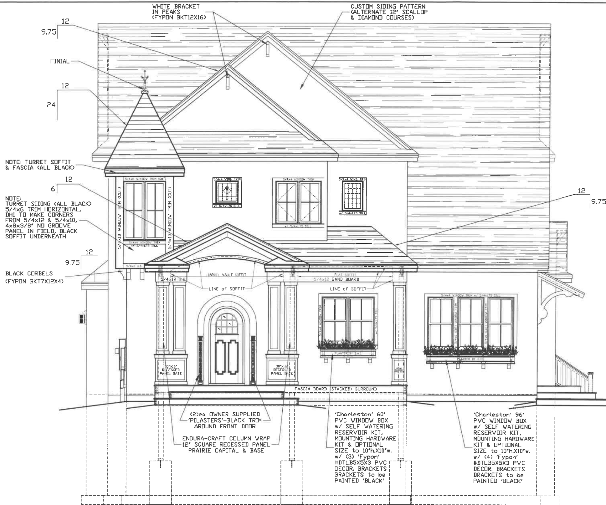
FRONT ELEVATION EAST ELEVATION
