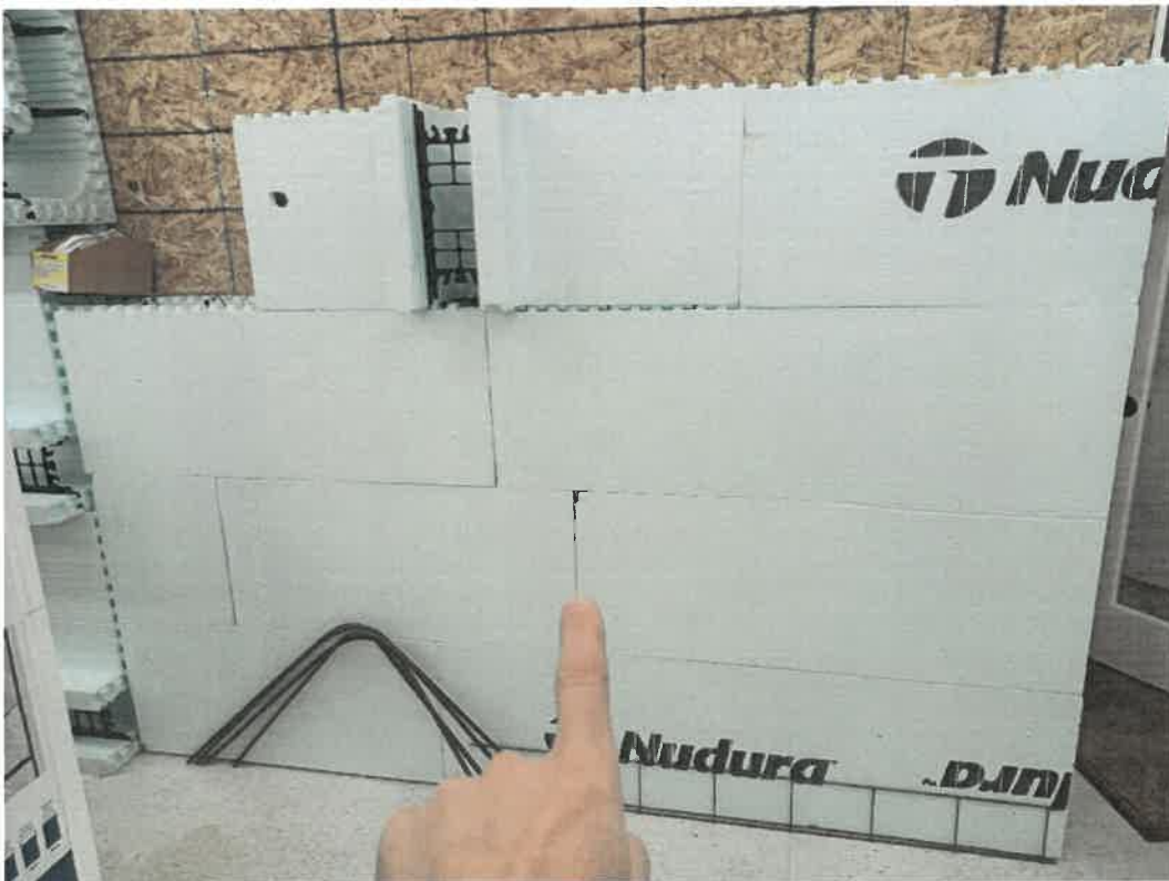
(The photo above illustrates damage caused by handling – not repairable)
