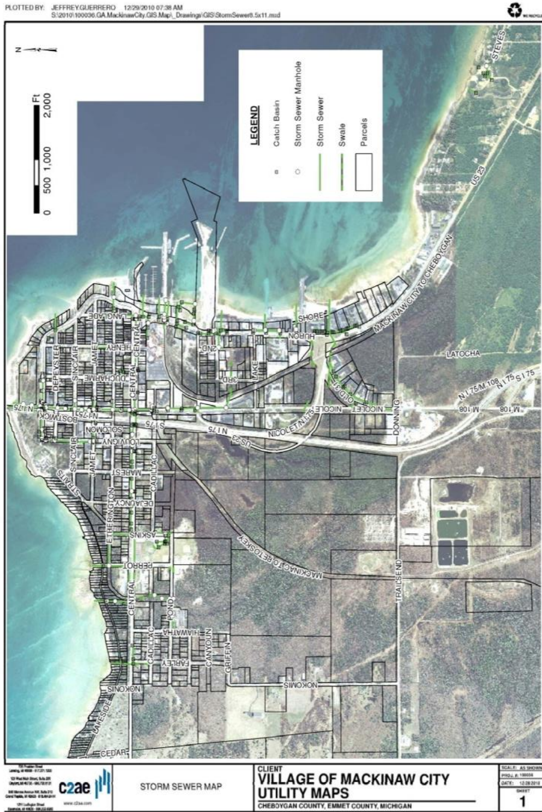
Figure 4-4 Village of Mackinaw City Stormwater Collection Map
