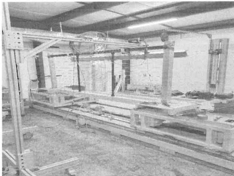
Photo No. 4 Test No. 2 – Uniform Load Test (Horizontal)
