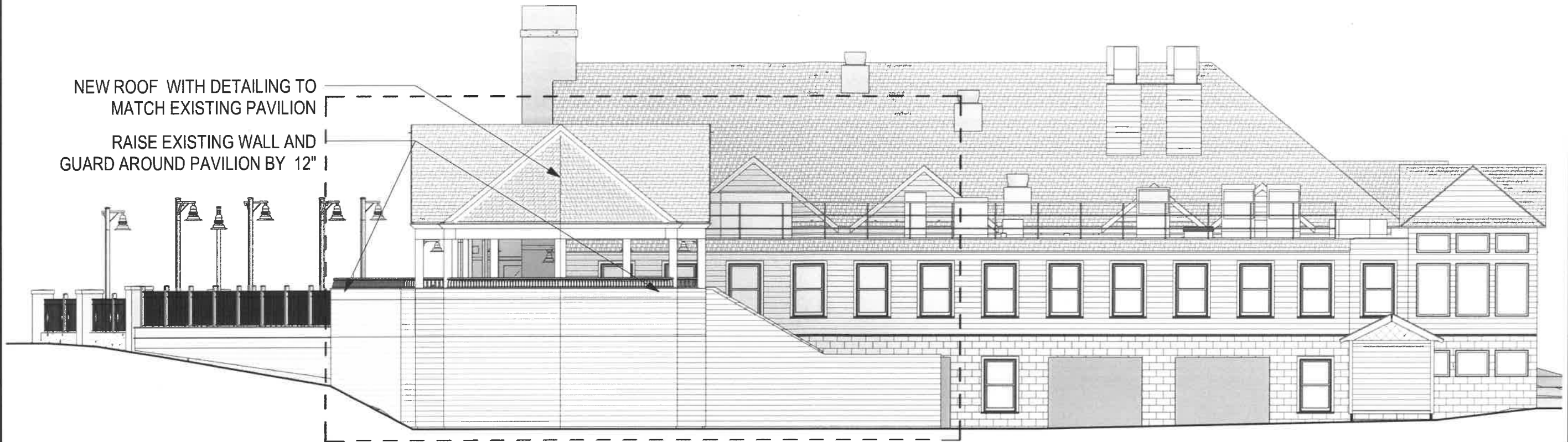
ELEVATION | BACK OF BUILDING
