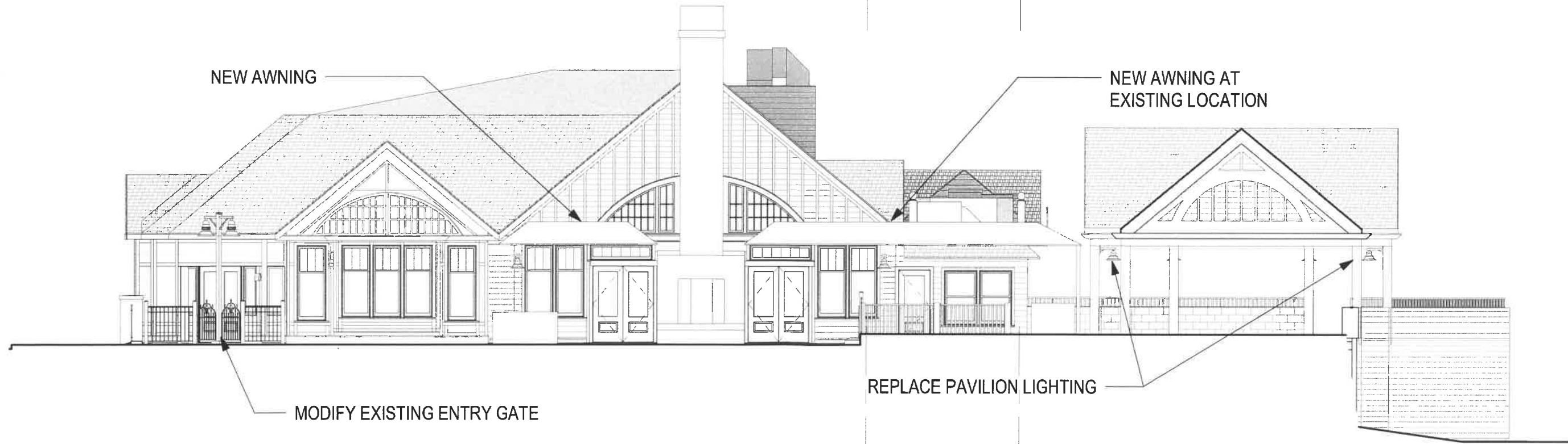
ELEVATION | FACADE MODIFICATIONS
