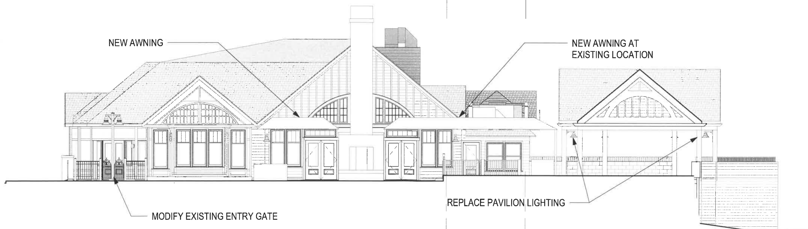
ELEVATION | FACADE MODIFICATIONS 1" = 10'-0" SCALE
