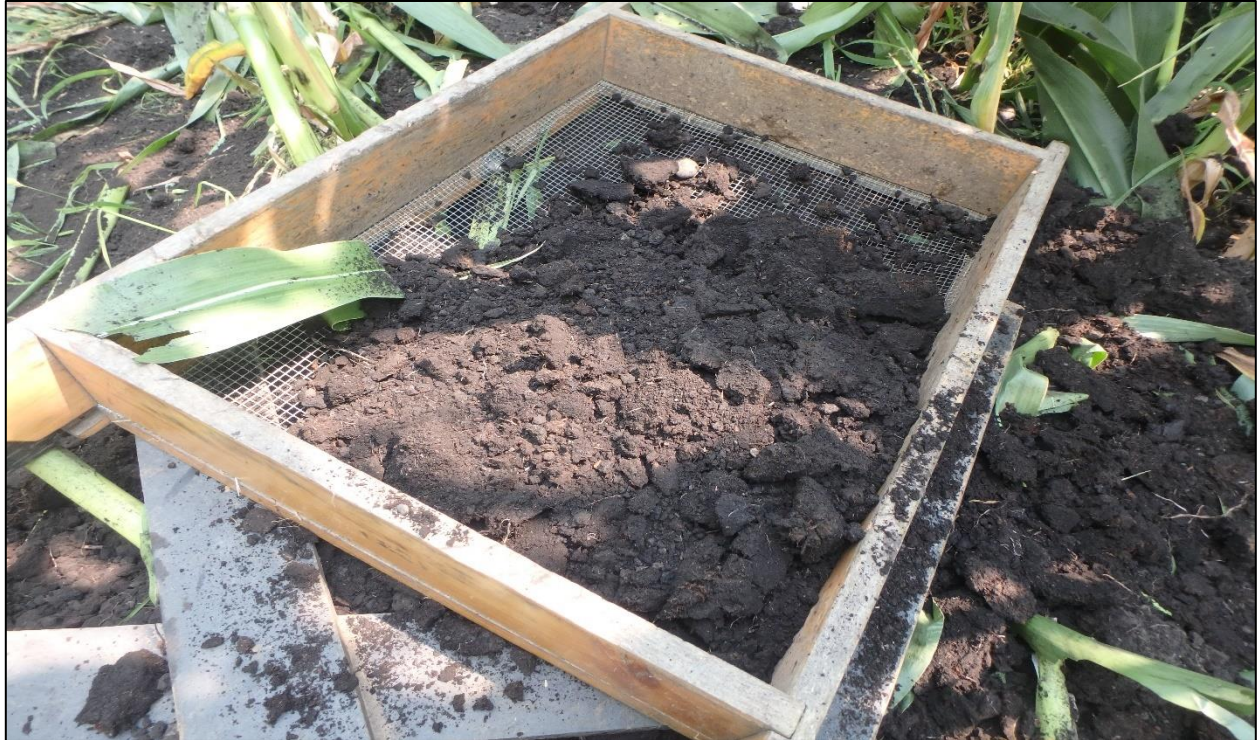
Photo 16. Detail of soils excavated from SP16 (2017), showing peats with silty-sands.
