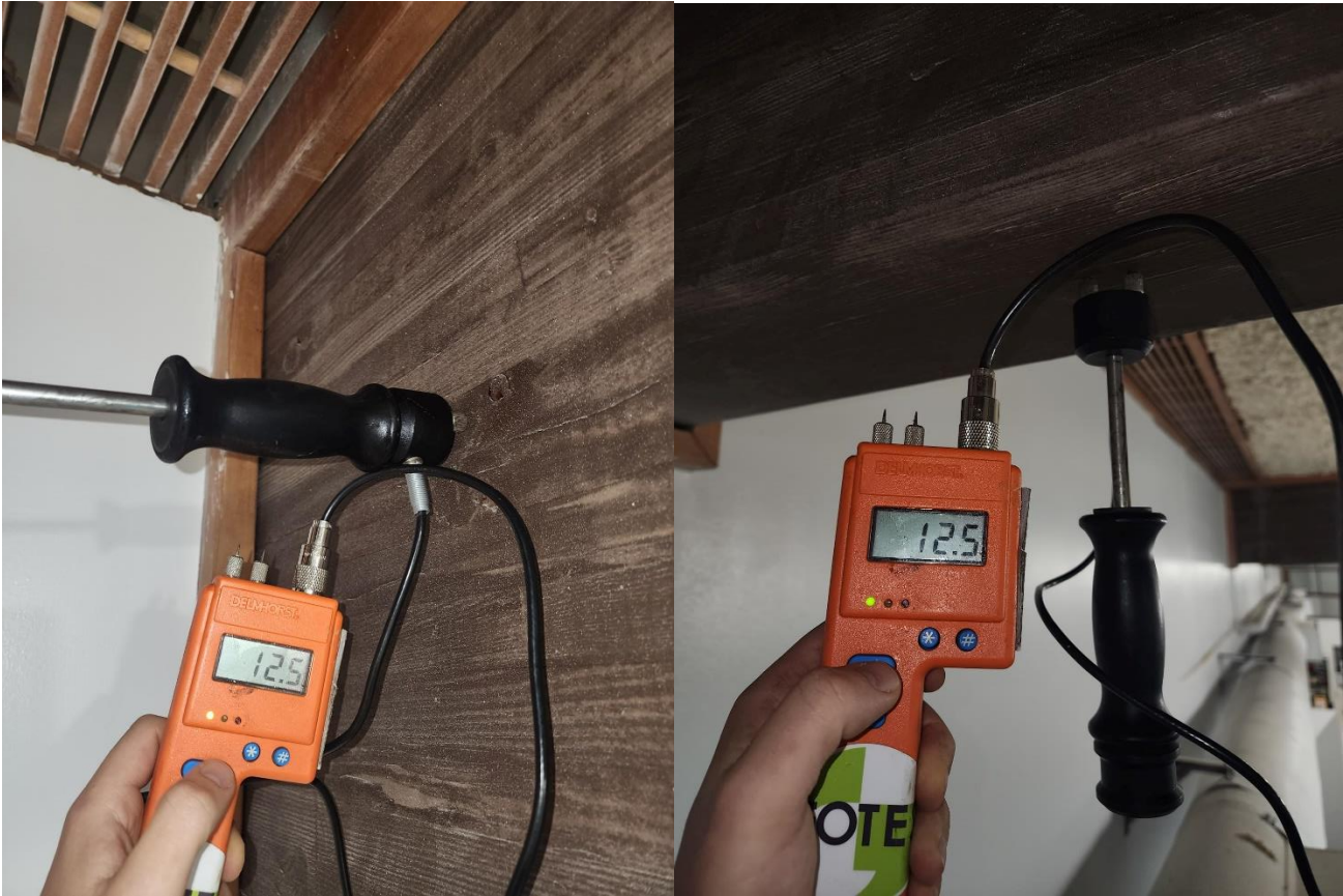
Figure 1: Beams were measured in two locations on the sides of the beams and two locations on the bottom of the beam.
