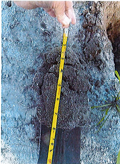
Apparent shell rock fill material placed in center of lot and around existing trees
