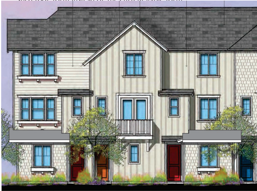
Replace low slope gable roofs with shed roofs
