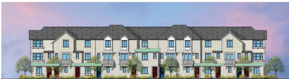
Replace low slope gable roofs with shed roofs Consider wider shed roofs to create stronger "entry porch" feel
