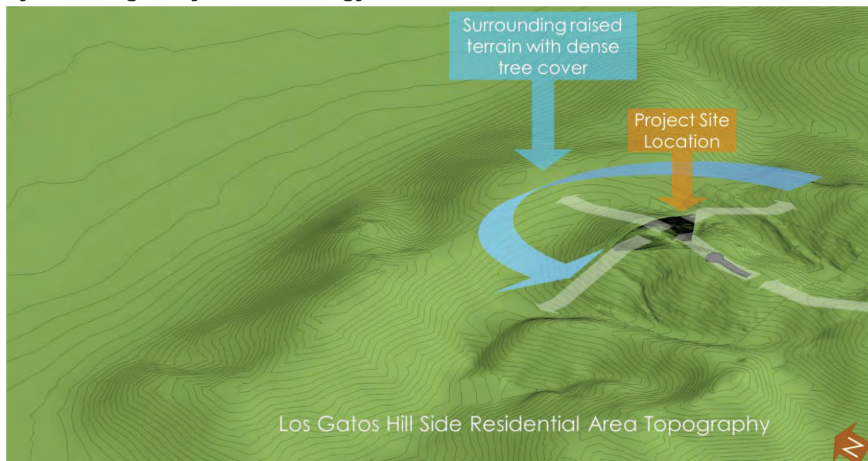
Figure 1 Site and Neighborhood Terrain was modelled based on topography drawings and Google Earth
