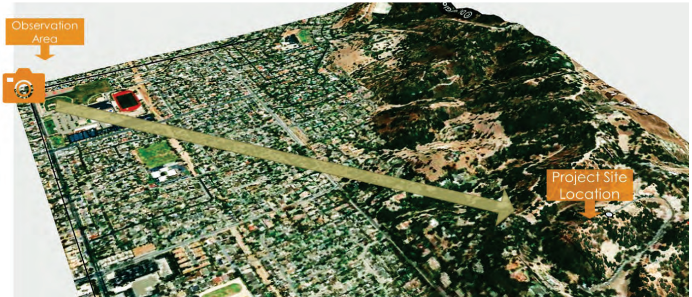
Figure 2: "Sketchup" and Google Earth were used to configure the location and altitude of the View angles.
