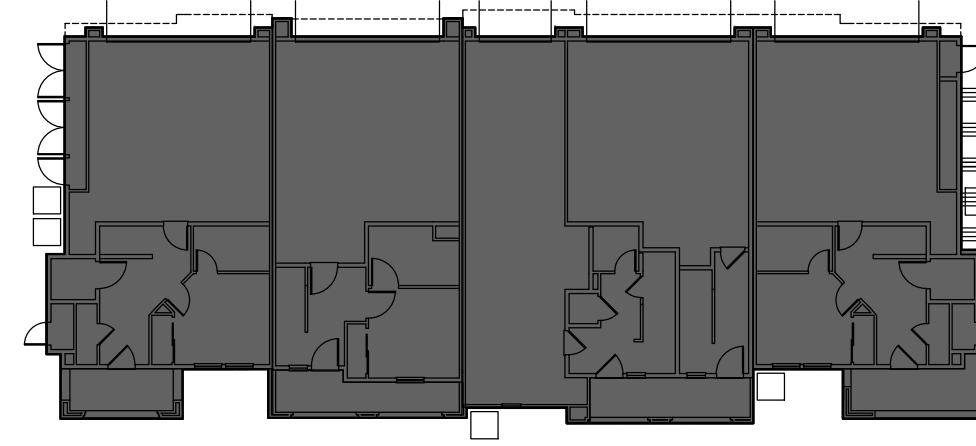
5 UNIT ALT BUILDING-WRAPPED PORCH (1 BUILDING ON SITE) LOT COVERAGE AREA PER TOWN CODE CALCULATION = 4,284.14 SQ. FT. x 1 BUILDING = 4,284 SQ. FT.
