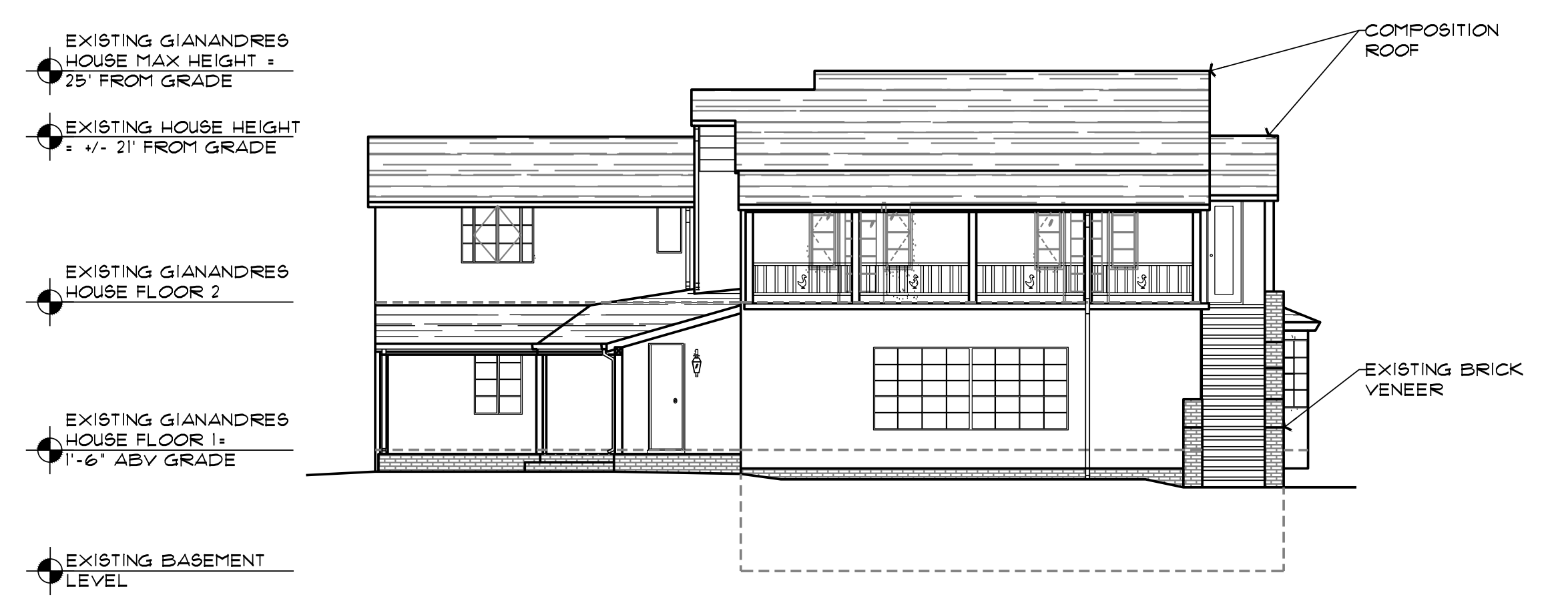
EXISTING SOUTH ELEVATION SCALE: 1/8" = 1'-0"
