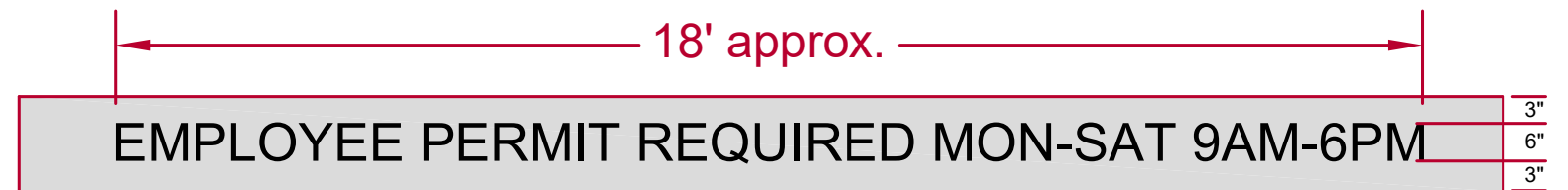
Detail A - Employee Permit Parking Stencil
