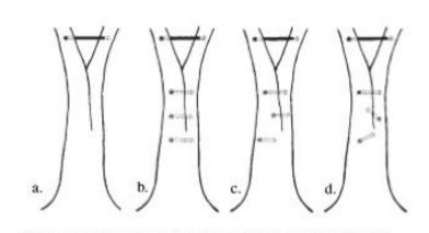
Figure 1. Bracing system types: (a) Single, (b) Parallel, (c) Alternate, and (d) Crossing *Credit: Tree Care Industry Association*
