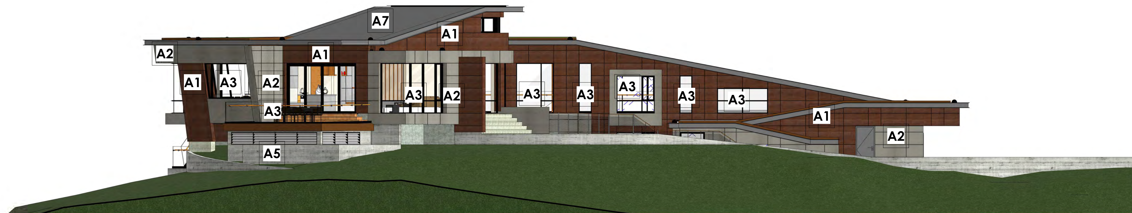
4 West Elevation with Exterior Materials Identified 1/8" = 1'-0"
