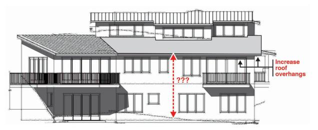
B. Extend the balcony across the facade connecting the currently proposed balcony and deck. The middle floor has been cantilevered out 18" to between the balconies to break up
