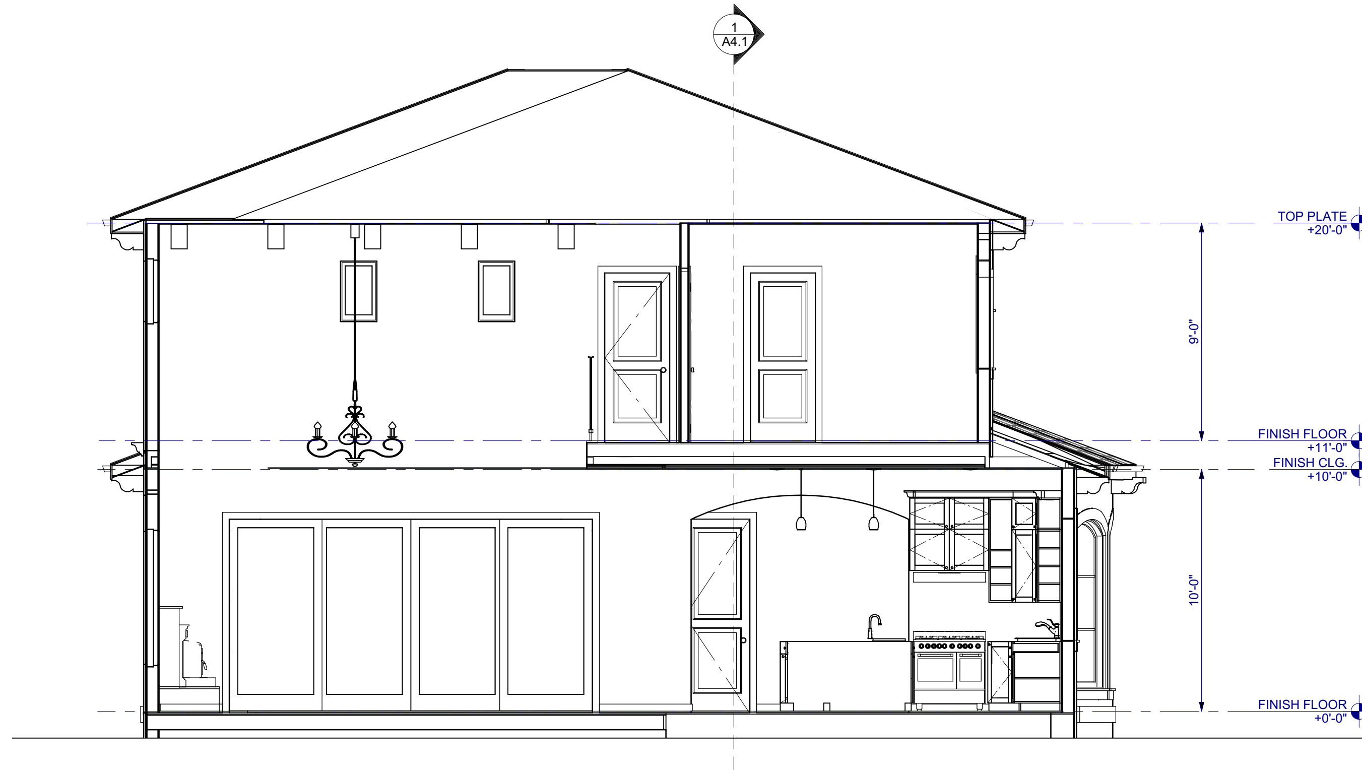
2 BUILDING SECTION Scale: 1/4"=1'-0"
