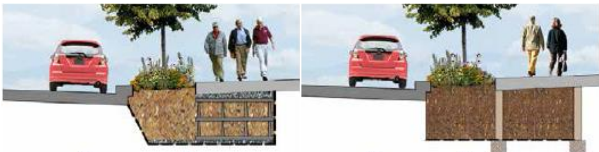
Figure 2-2 Stormwater tree well filter conceptual examples: modular suspended pavement system (left), column suspended pavement system (right). (Courtesy of City of Philadelphia Water Department)
