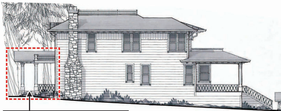
Porch entry extension too long and not characteristic with the style
