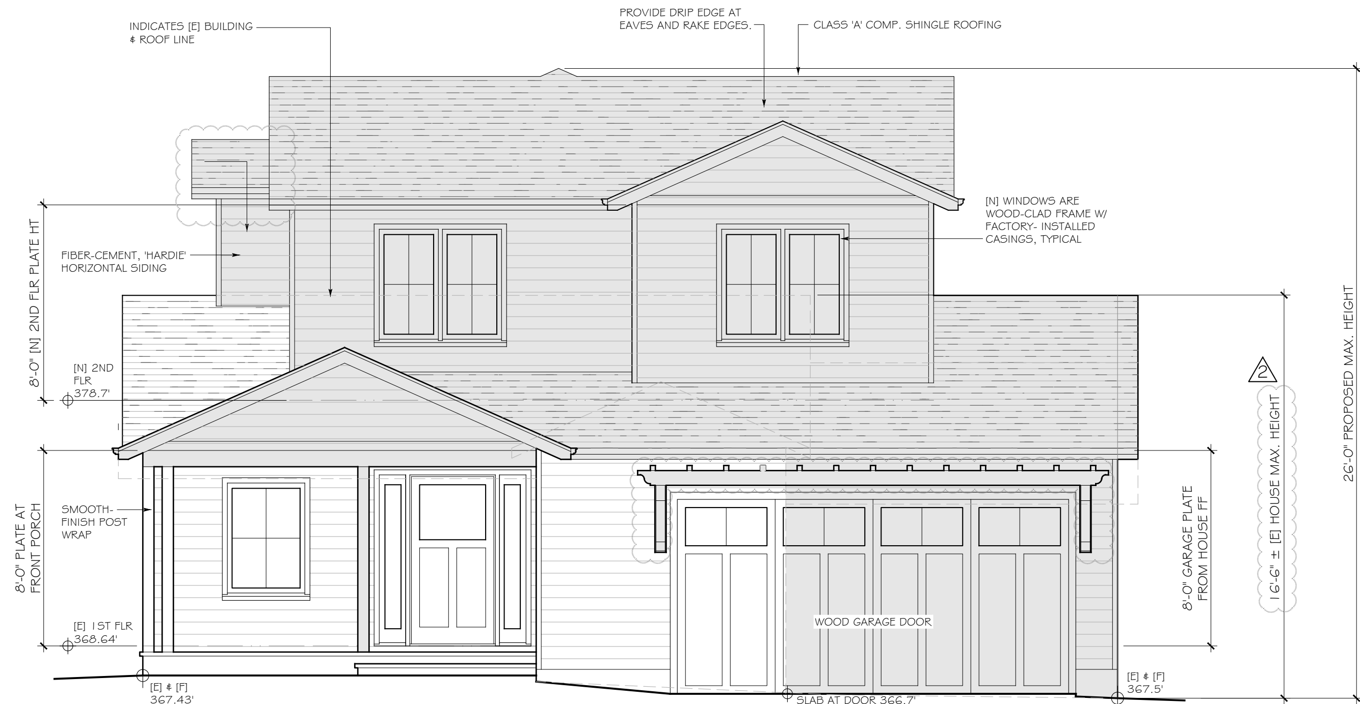
FRONT (EAST) ELEVATION
