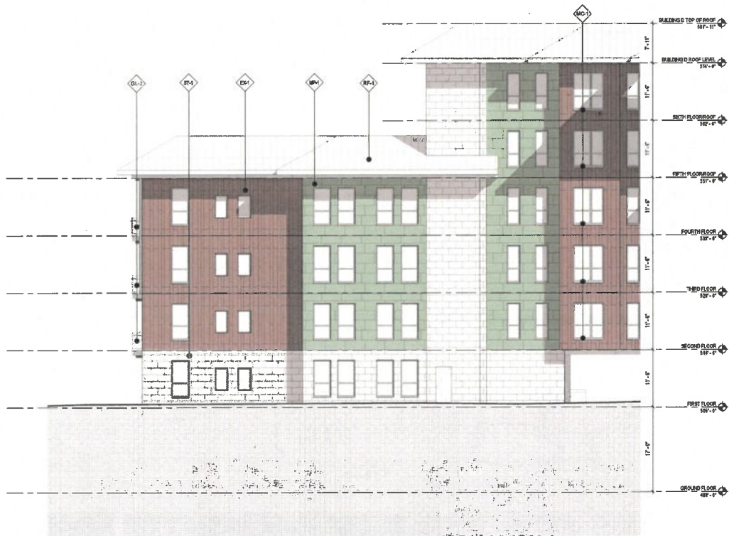
2 VILLA D NORTH-WEST ELEVATION 1/8" = 1'-0" NOTE: SEE SHEET A201 FOR MATERIAL BOARD
