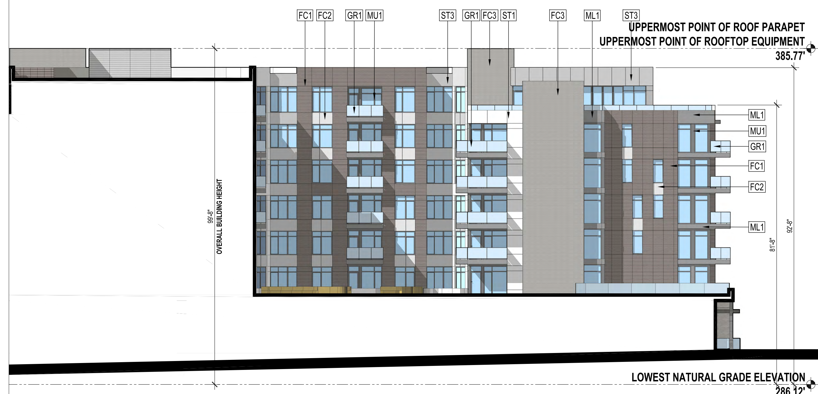
3 COURTYARD EAST ELEVATION 1/16"=1'-0"
