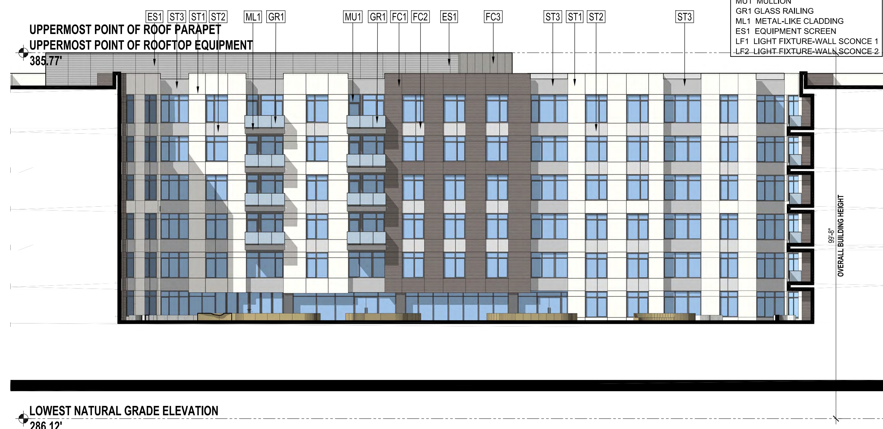
4 COURTYARD NORTH ELEVATION 1/16"=1'-0"
