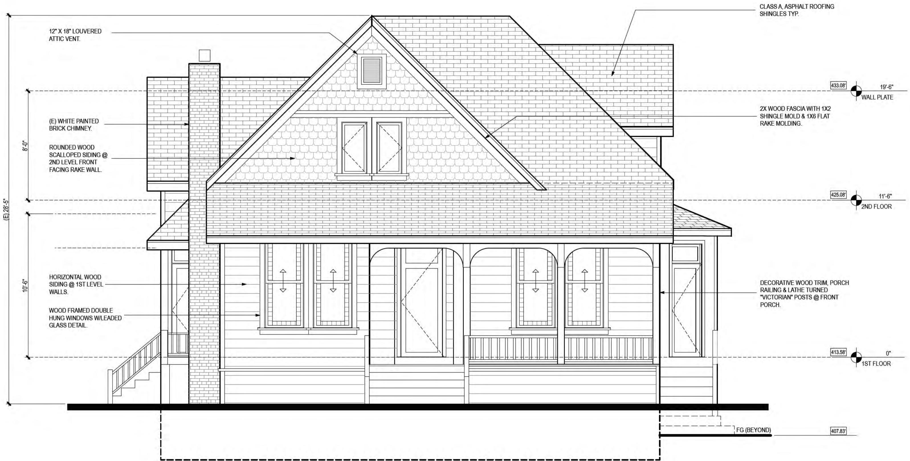
1. EXISTING FRONT ELEVATION (SOUTHWEST) BACHMAN AVENUE SIDE 1/4" = 1'-0"
