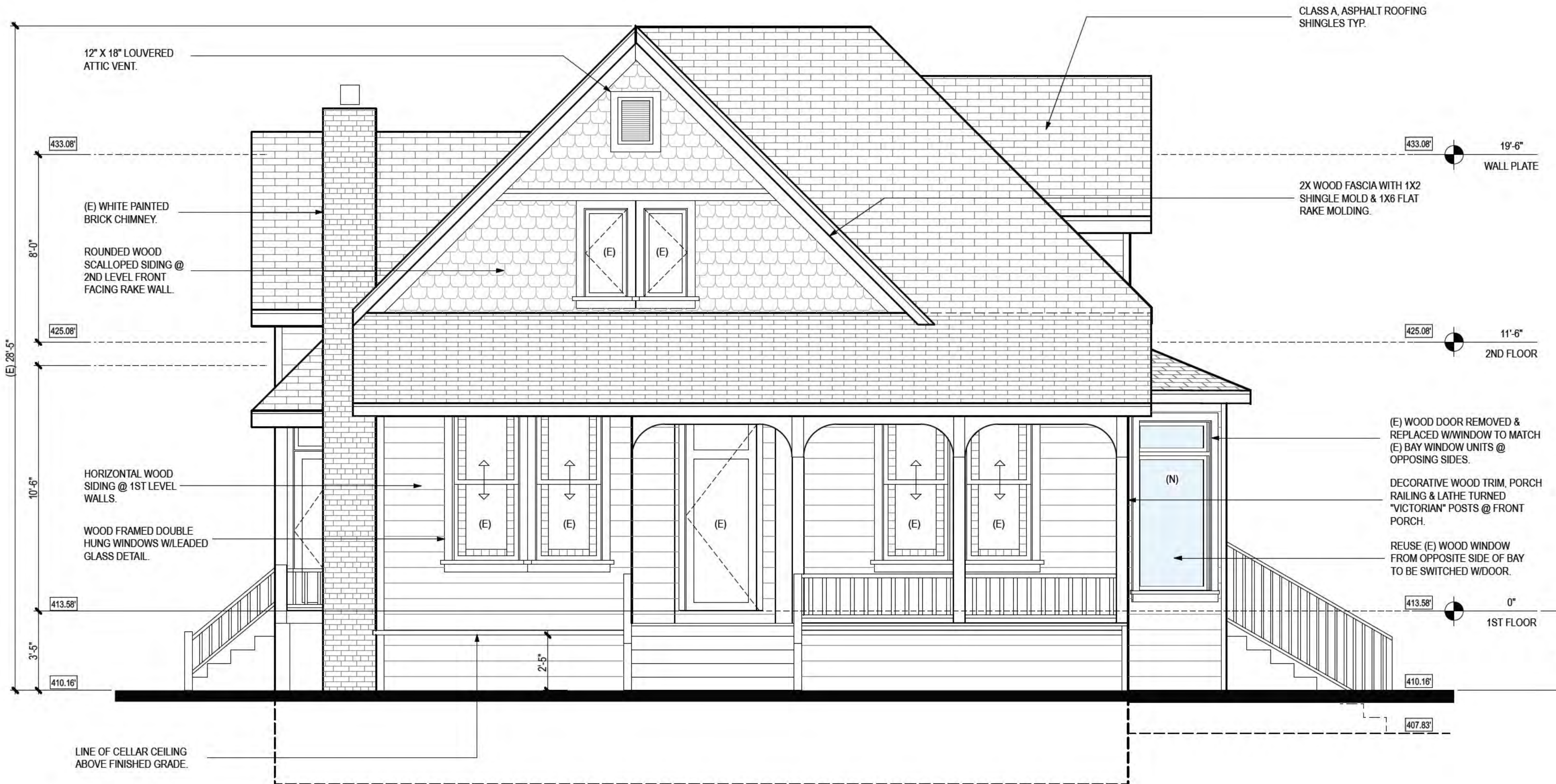
1. EXISTING FRONT ELEVATION (SOUTHWEST) BACHMAN AVENUE SIDE 1/4" = 1'-0"
