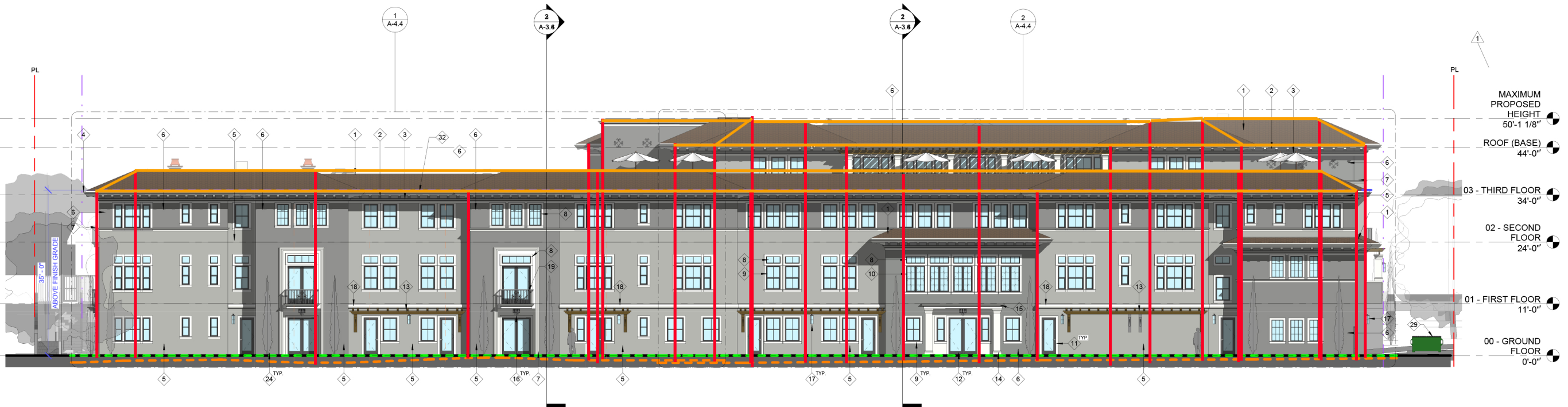
2 EAST - FACING RESIDENTIAL ELEVATION 3/32" = 1'-0"
