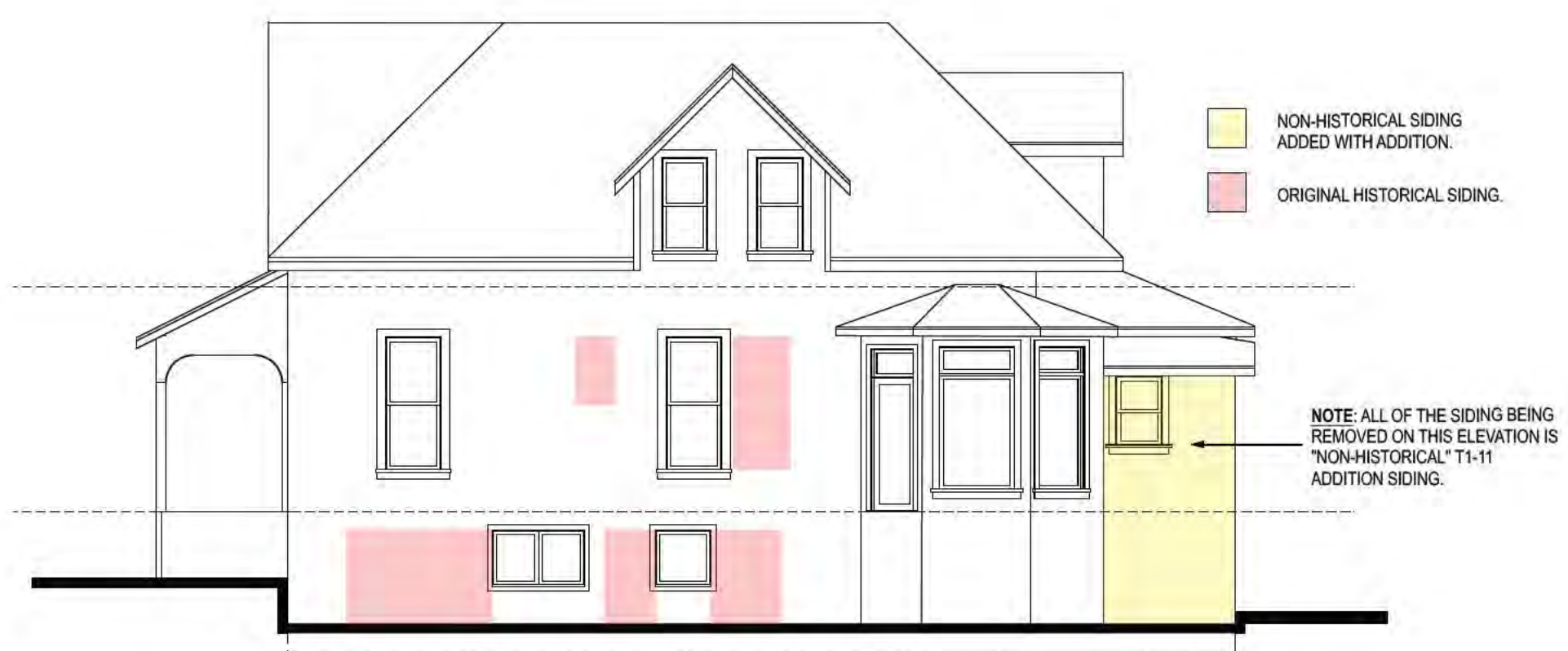
905 SF OF EXTERIOR WALL. 176 SF OF EXTERIOR WALL SIDING REMOVED. (19%) NOT FACING A PUBLIC STREET. EXISTING RIGHT SIDE ELEVATION (NORTHEAST) 1/8" = 1'-0"
