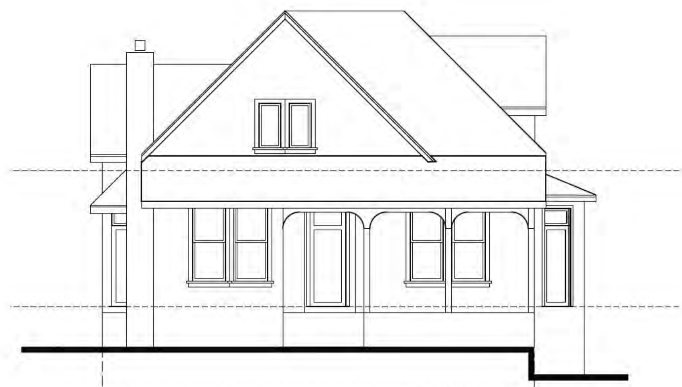
593 SF OF EXTERIOR WALL SIDING. 0 SF OF EXTERIOR WALL SIDING REMOVED. (0%) FACING PUBLIC STREET. EXISTING FRONT ELEVATION (SOUTHWEST) 1/8" = 1'-0"
