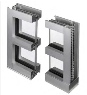
SF-1: ALUMINUM STOREFRONT MFG: KAWNEER (BASIS OF DESIGN) PRODUCT: TRIFAB VERSAGLAZE 451, 2"X 4 1/2" FINISH: ANODIZED ALUMINUM(MATCH EXISTING)
