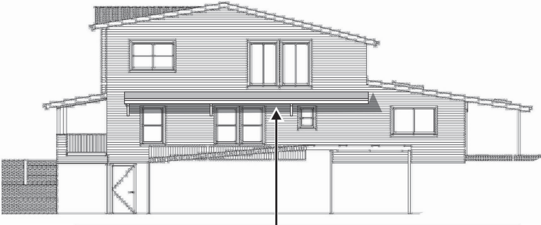
Add shed roof to be consistent with Residential Design Guideline 3.3.3
