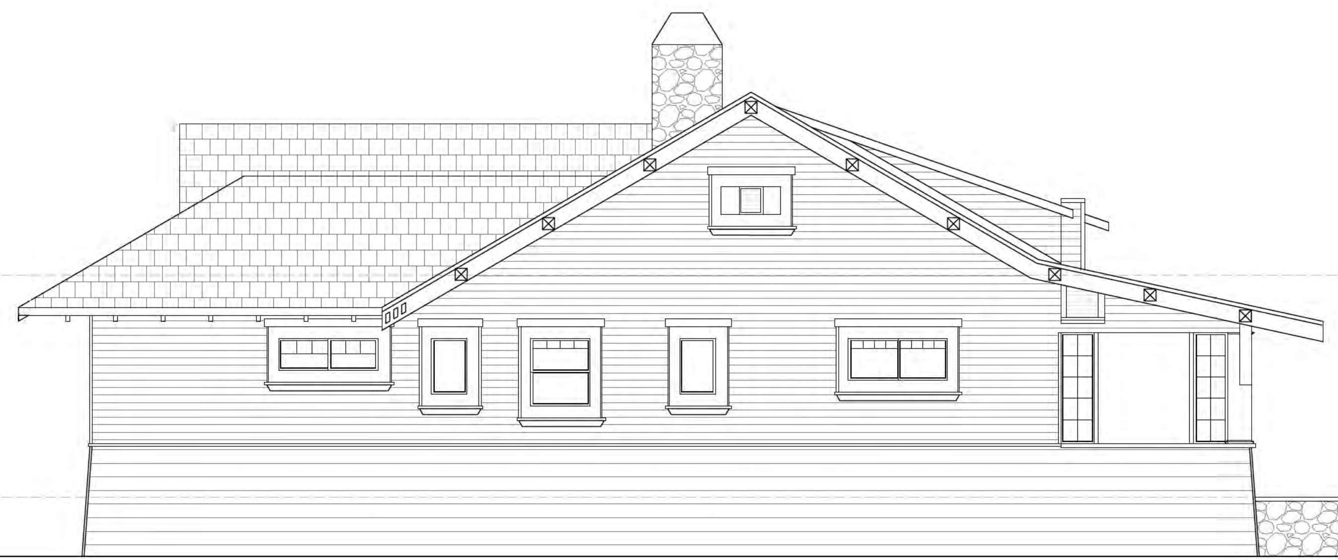
EXISTING LEFT-SIDE ELEVATION 1/4" = 1'-0"
