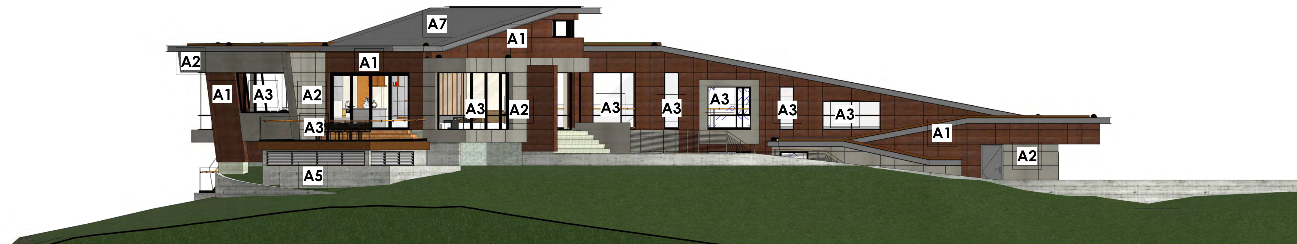
4 West Elevation with Exterior Materials Identified 1/8" = 1'-0"
