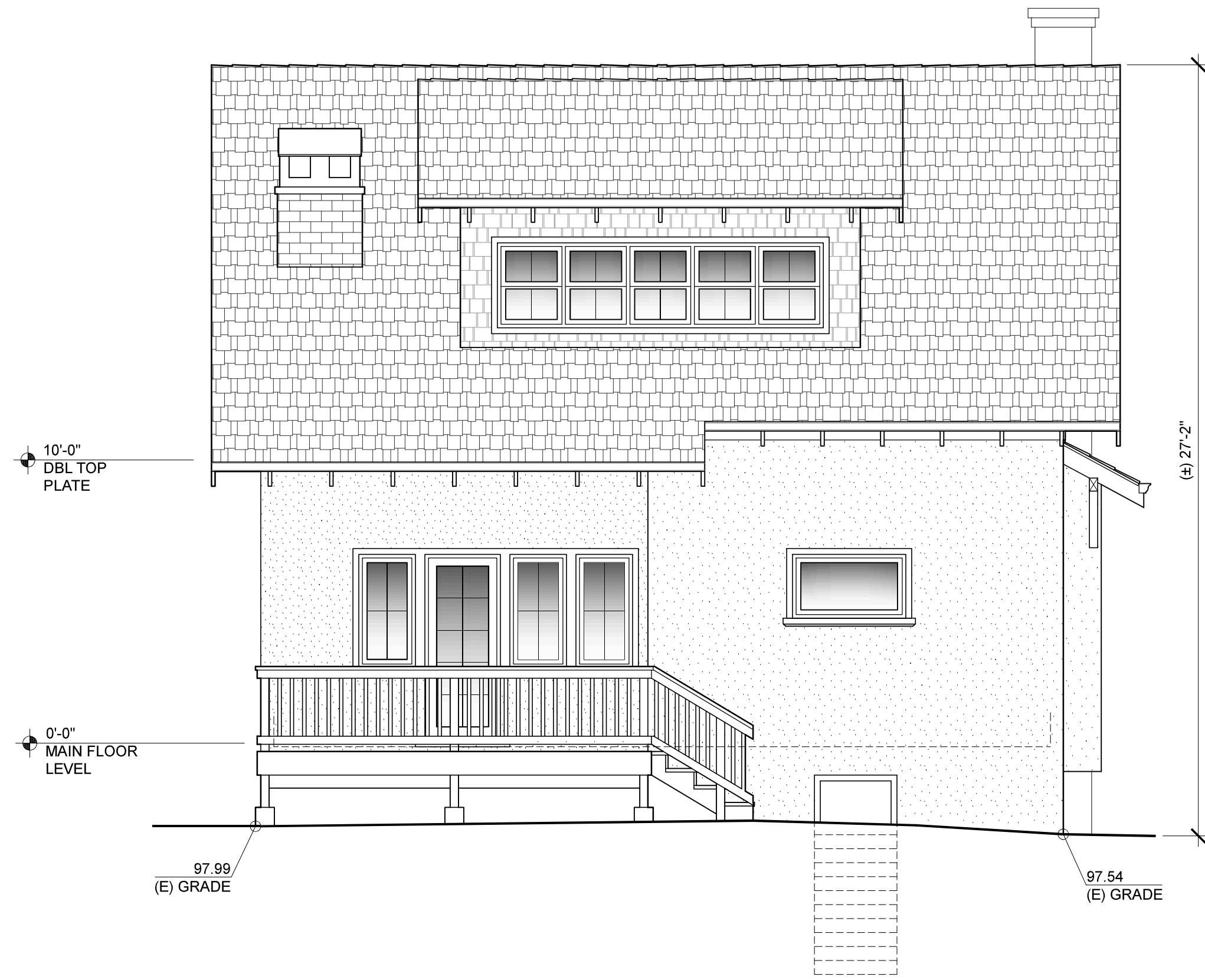
EXISTING RIGHT INTERIOR SIDE / WEST ELEVATION
