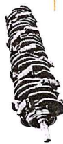
Bite Limiter rotor special steel limiter rings control the depth of cut
