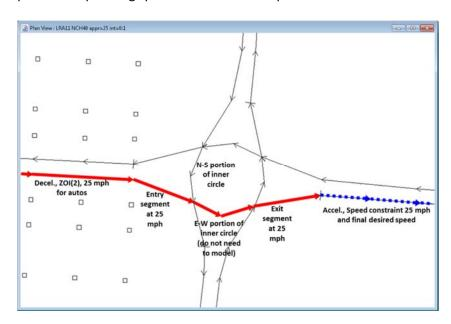
A roundabout with a two-lane inner circulatory road may be modeled essentially the same way as described for the one-lane inner circulatory road.
