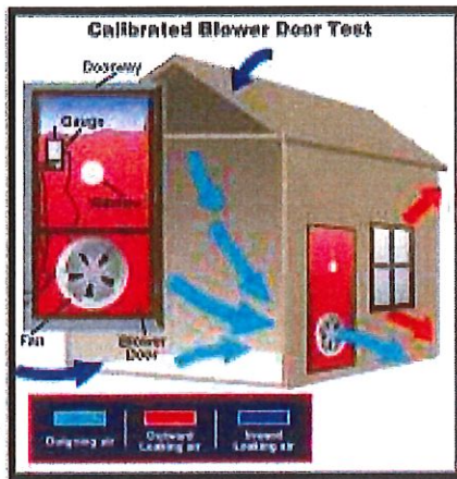
Figure 1 Blower door test (Source: Technically Speaking: What the Blower Door Test Tells You / Building Performance Institute, Inc. ( bpihomeowner.org )).
