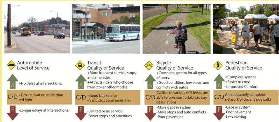
Figure I-2: Transportation Levels of Service
