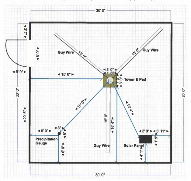
Note: guy wires are not necessary if the concrete anchor pad for 10-m tower is 36"x36"x48" in solid soil. Sites without guy wires can cover a smaller area footprint (< 30'x30' site). Sites near the coast that may experience ≥ 110 mph winds due to hurricanes will need additional guy wire support and thus will require the 30'x30' footprint.
