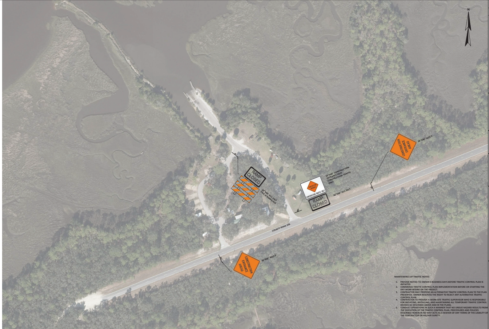
TRAFFIC MAINTENANCE PLAN SCALE: 1"=60'
