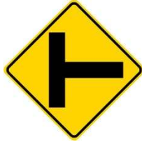
Figure 4. Side Road Advanced Warning Sign (MUTCD W2-2R)
