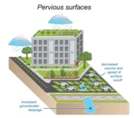
Pervious 'soft' surfaces (green roofs, rain gardens, grass paver parking lots, and infiltration trenches) decrease volume and speed of stormwater runoff. The slowed water seeps into the ground, recharges the water table, and filters out many pollutants and sediment before they arrive in downstream waters.
