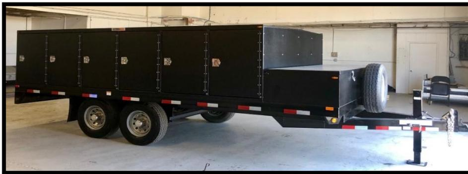
**72 MVB3X Capacity Trailer with six compartments per side**
